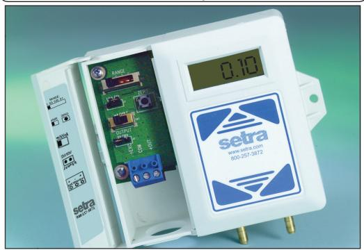
ers Systems 260 pressure transducers sense differential or gauge (static) pressure and convert this pressure difference to a proportional electrical output for either field selectable unidirectional or bidirectional pressure ranges. The 260 Series is offered with field selectable high level analog outputs of 0 to 5, and 0 to 10 VDC, or 4 to 20 mA.
